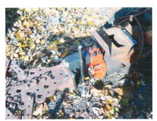
To attach your home grown or "Gravely" attachment to the new Non-powered adapter, use four 1/2' bolts of sufficient length as needed. If your attachment has a 3/8 bolt or a cast lug that held back the advance casting PTO shaft, clearance is provided in the
