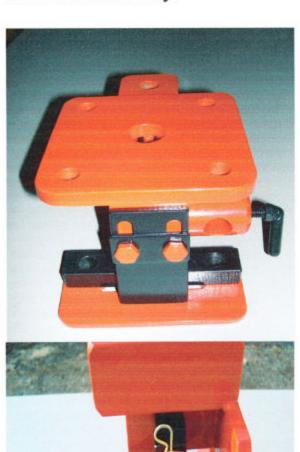
Bolt the slotted push bar using the provided 3/8" X 3/4" grade 5 hex bolts and the small 1/8" thick 2-hole tie plate to the bottom side of the Weldment into the 2 tapped holes. Apply a little oil or light grease before inserting bolts into threads. Leave these bolts only snug till final adjustment to your machine. The 2-hole tie plate provides a better locking grip for the push plate than simple washers.
