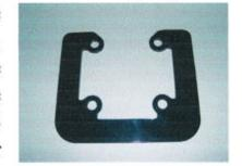
We offer an optional modified hex stud (with a shorter hex portion) to allow the 4-stud reinforcing retainer plate surface to fall behind the quick hitch casting surface and therefore getting the 4-stud reinforcing retainer plate back behind the travel of the teardrop shaped tilt limit plate of the snow blower or similar attachment.
