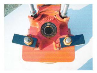
The provide "C" shaped 2 hole push plate (also called 2-stud reinforcement retainer plate) is attached to the lower two double ended Q H studs (not supplied with this kit) of your quick hitch. Our optional "horseshoe" shaped 4-stud reinforcement retainer plate
